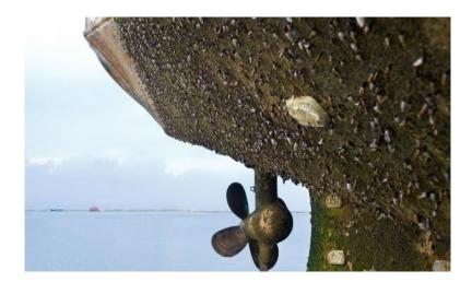
Figure 4.4: Ship's bio-fouling by marine organisms
