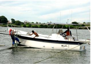
Mauritius and the Overseas Fishery Cooperation Foundation (OFCF) of Japan, the MEXA 1 underwent a major overhaul of fishing boat MEXA 1. The cost of improvement works was funded by the OFCF, under close supervision of OFCF experts. The overhaul has enabled fixing of new fishing equipments. The rehabilitation work consisted of change of fish hold, self bailing deck, erection of cabin, hydraulic steering equipment, line hauler, navigation lights, etc.
