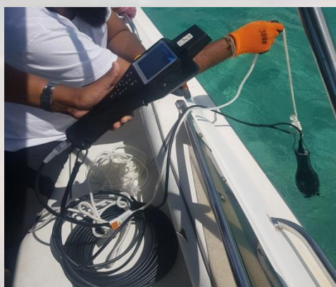
Figure 22 - In-situ measurement of seawater quality using multiparameter meter
