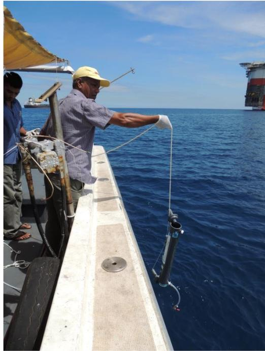
*Figure 15 - Collection of seawater sample using Niskin water bottle*
